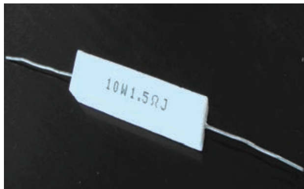
Fig.2 A cement wire wound resistor as a switcher
